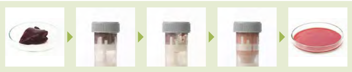
Dispersion example in a DT-20 tube: liver
